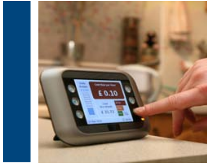
Smart meter display in kitchen
